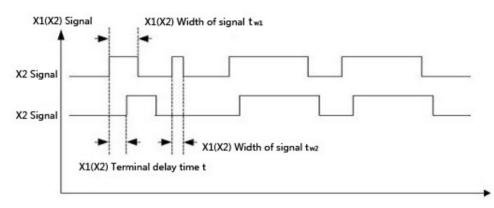
Figure 6-14 X1/X2 terminals delay
